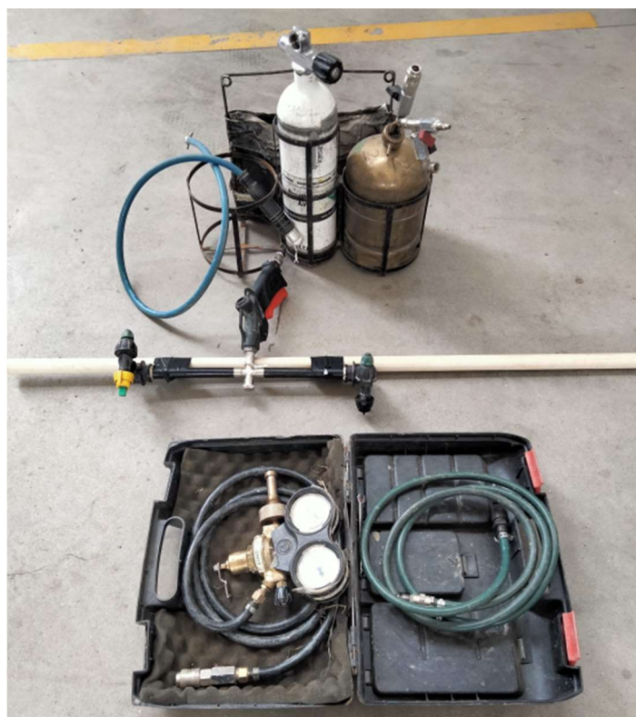
Photo - 2 equipment: air compressed, canister for mixture, pressure gauge, Nozzle (one of the two nozzles in photo was closed)
