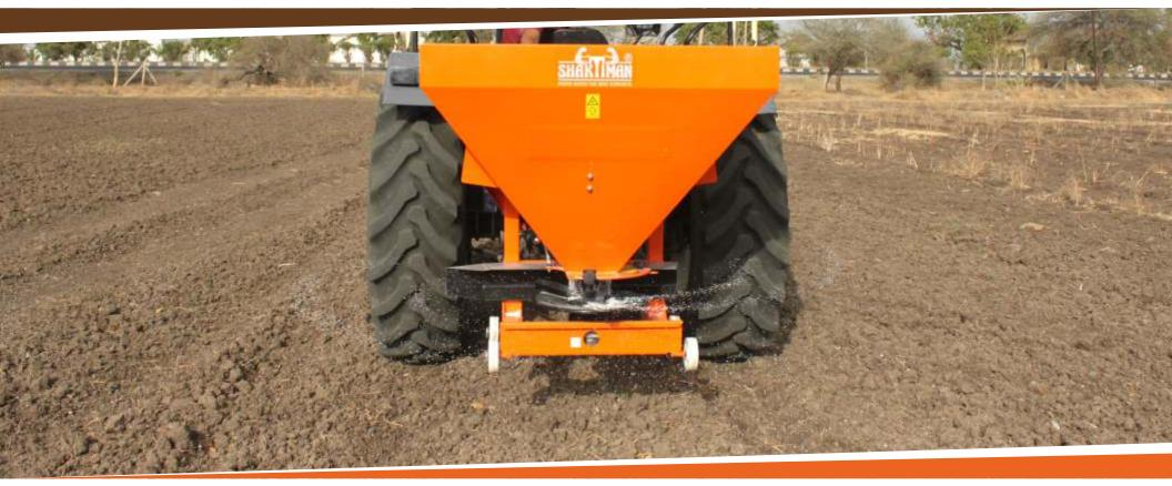
**SHAKTIMAN** Square Fertilizer broadcaster is a machine with square shape Hooper, Spreading disc system with four blades, ideal for granular or crystalline fertilizer. Its unique distributing system ensures uniform spreading of fertilizer over greater distance.
