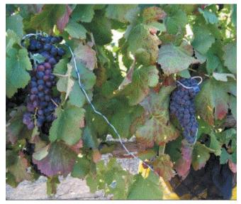
Figure 10. Measurement of the temperature of berries using captors which are inserted between the skin and the pulp. Data loggers permit the automatic acquisition of temperature values. Cultivar Syrah (South Africa, vineyard in Stellenbosch, at the ARC-Infruitec-Nietvoorbij). The direction of the rows was north - south (Deloire & Hunter, 2005).
