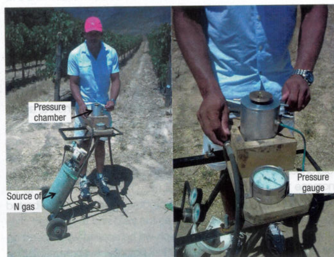
FIGURE 1. Example of a pressure chamber used to measure leaf water potential. (Photo from L'Ormarins vineyard)
