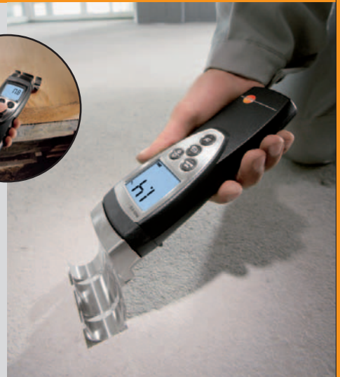
Fast and easy – moisture checks on screed. Measuring several points across a surface ensures more security.
