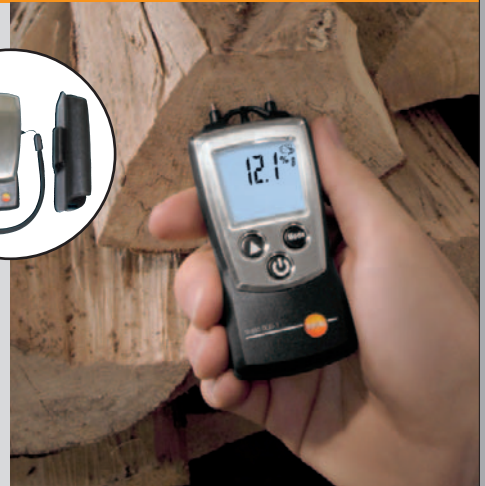
Checking wood moisture
