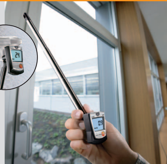
Flow velocity measurement at nontight windows
