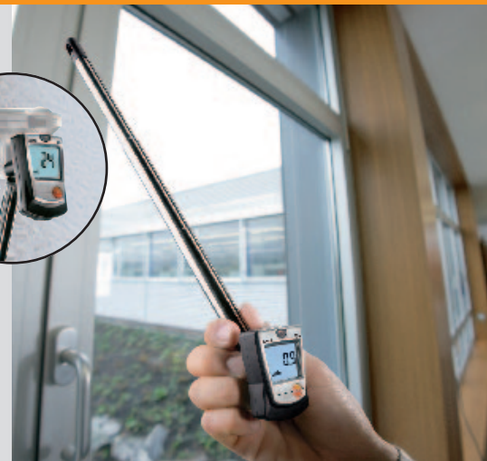
Flow velocity measurement at nonglazed windows
