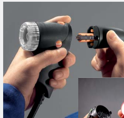
Exchanging probe shaft
