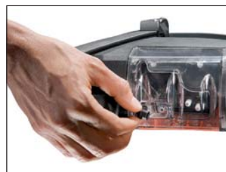
Continuous condensate drain-off for long-term measurements
