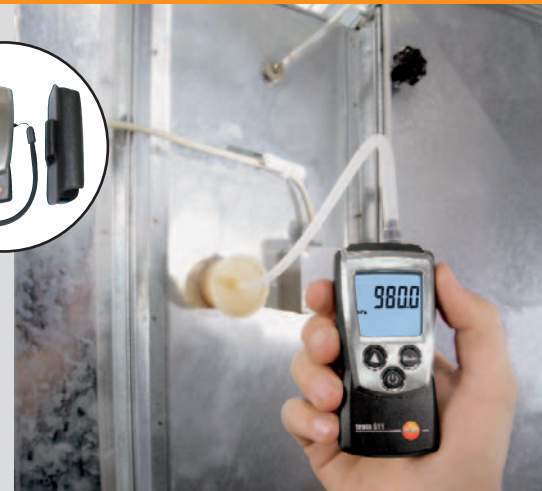
Absolute pressure measurement to determine absolute pressure compensation when measuring flow with a Pitot tube
