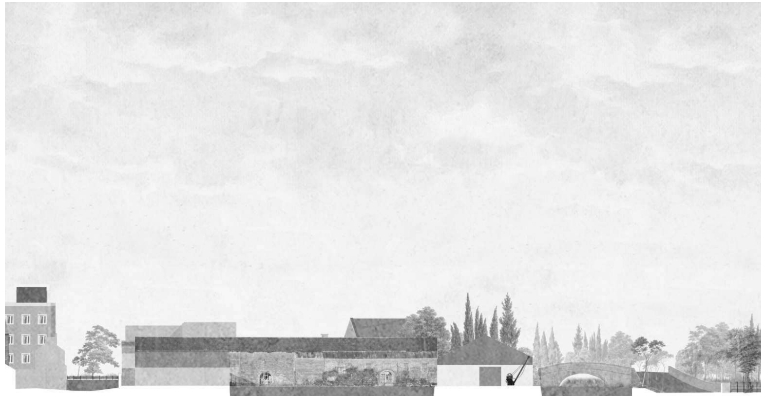
A section of the current condition showing the Basin, Canal Spur and Embankment.
