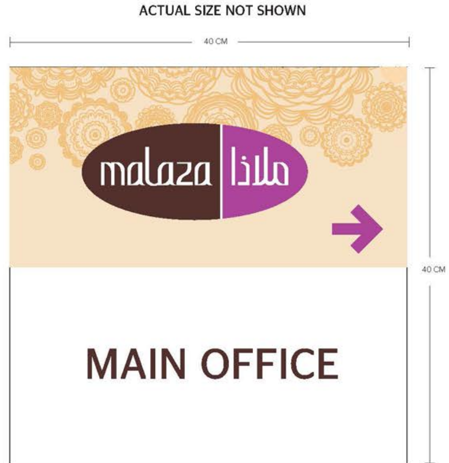
MAIN OFFICE SIGN ( DIMENSION: 40 CM W X 40 CM H ) ACRYLIC THIN SHEET IN 5MM PRINTED
