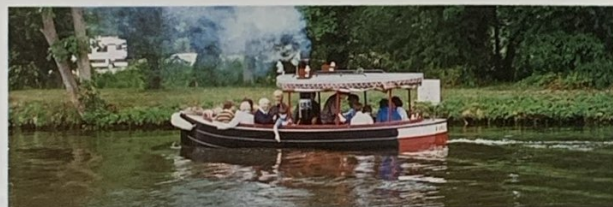
Fireweed, a coal fired steamboat built in 1988 by Concoform Marine to special order.
