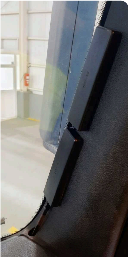
Internal LTE and GPS antennas in the cabin
