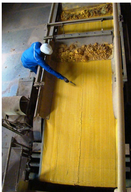
Figure 10. Production of yellow cake (filtration) in uranium mine and milling facility.
