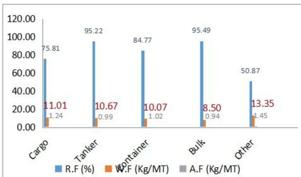
Figure 5. Relation among average reusable, waste and asbestos factor with LDT of EOL ships
