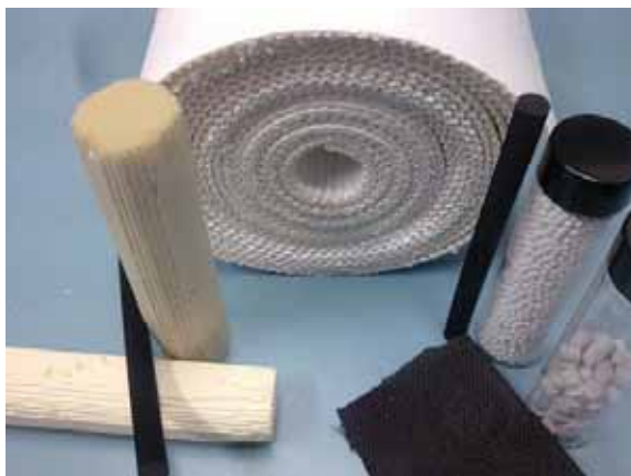
Figure 1.4: Illustration of a variety of adsorbent structures including (left to right): ceramic and carbon adsorbent monoliths, corrugated paper monoliths (centre), fabric adsorbent and conventional beaded adsorbents.
