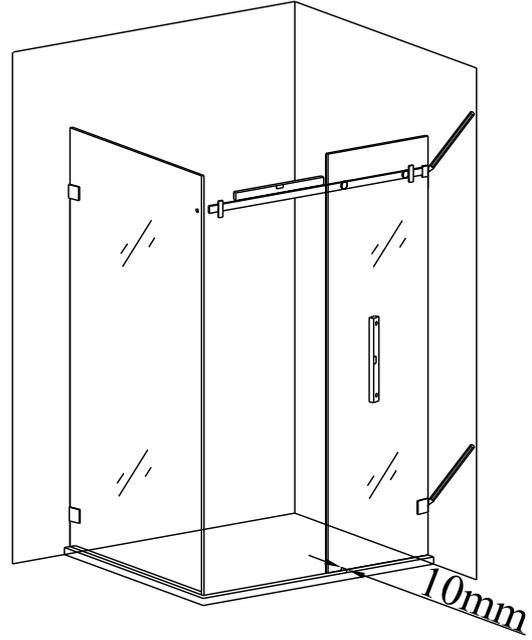
1. Put the fixing glass on the base stone. The distance between them is 10 mm. Make them vertically by spirit level, marked by pencil, then take off the fixing glass.
