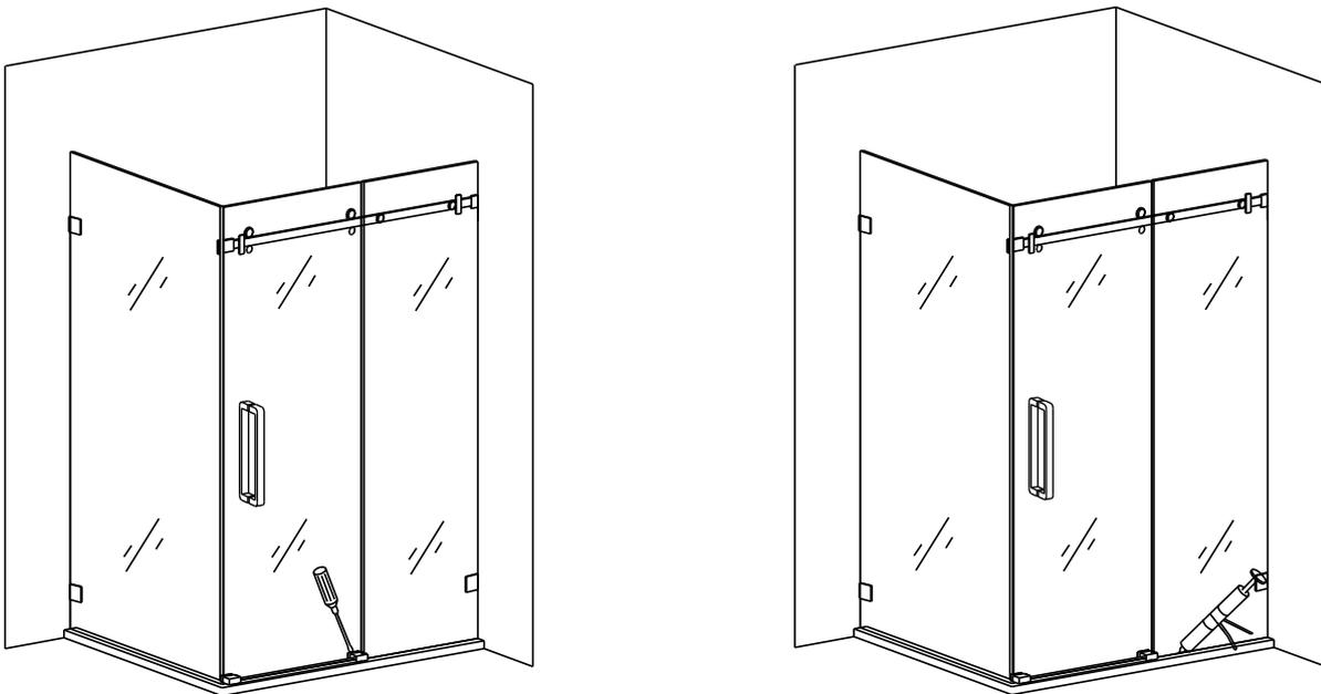
1. Put the waterproof bar on the base stone, locked it tight with flate tapping screw M4×30.
