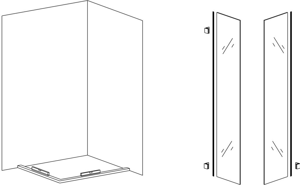
1. Select the installation position, put the base stone or tray to the position and measure it vertically by spirit level.
