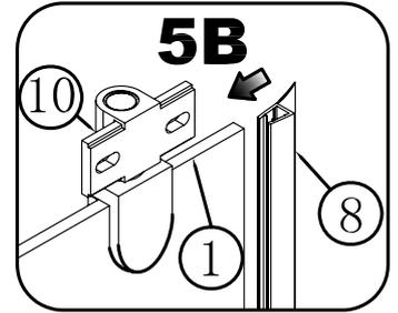
Install the vertical door seals along the whole height of the door, and fit the bottom drip strips in between.
