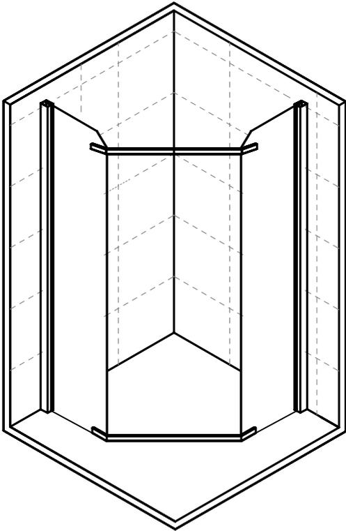
Fit metal brace to the top and bottom.
