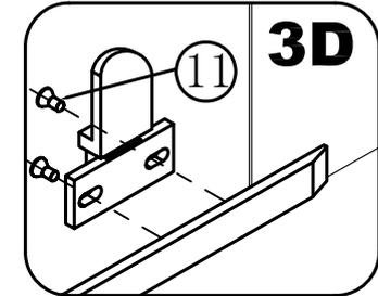
Install the door onto the bottom hinge.
