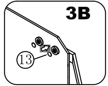
Install the bottom door hinge on the brace.
