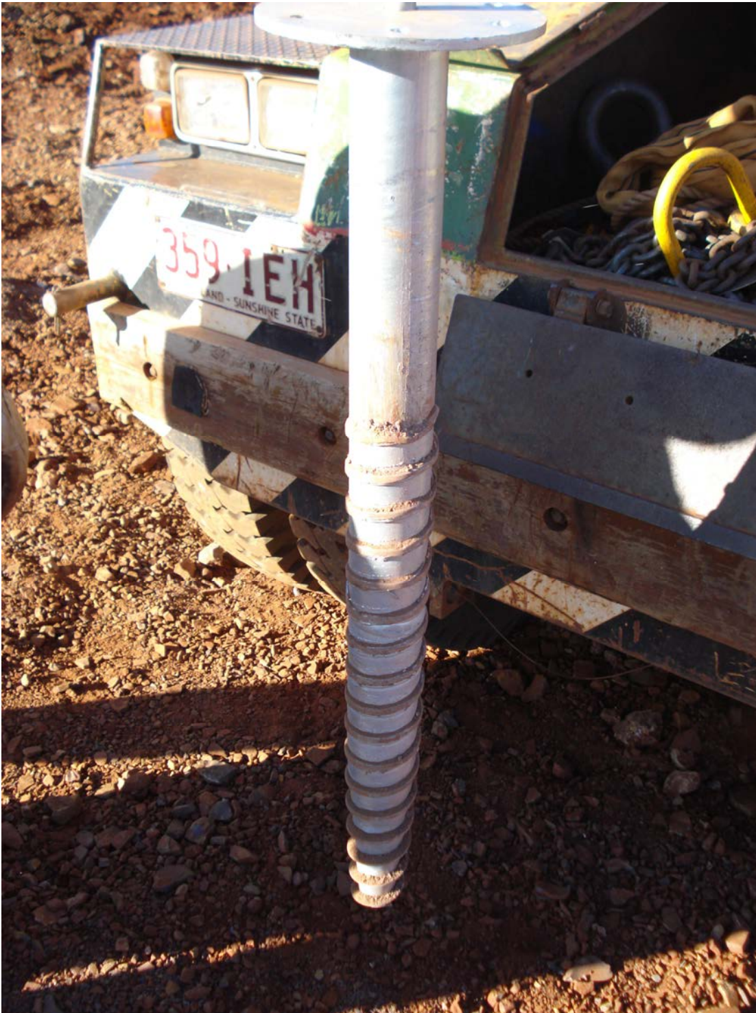
Photo 4. Screw after pullout Test 3 in rock, note deformation of upper threads.
