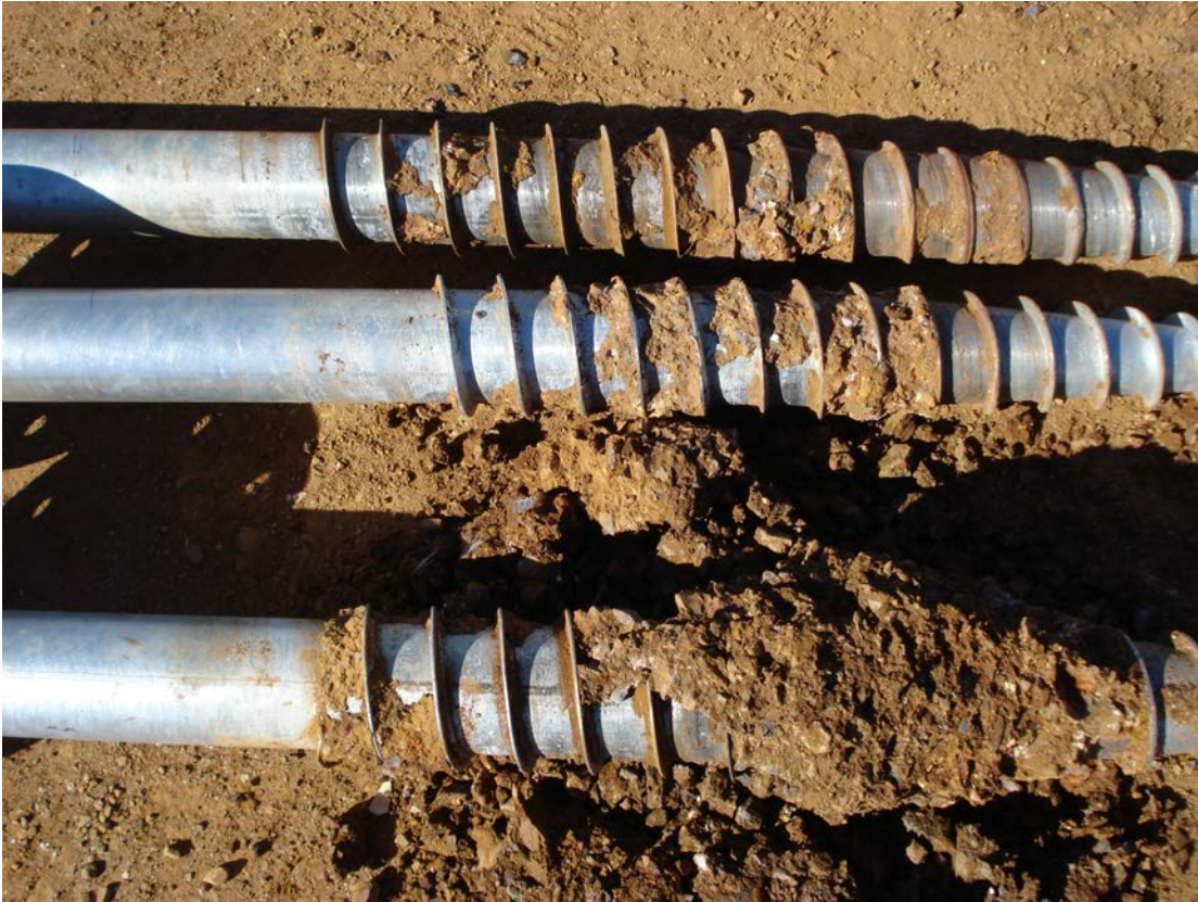
Photo 6. Ground screws after pullout in compacted fill
