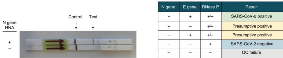
Figure 5: A result showing detection in both E and N genes is considered to be positive. A result showing at least one detection in either E or N genes is considered presumptive positive. A result showing detection in neither is negative, and it is considered failed if it also shows no detection in RNase P. Figure taken from journal “CRISPR–Cas12-based detection of SARS-CoV-2” by James P. Broughton et al., Nature Biotechnology
