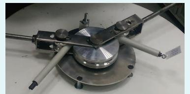
Sixty seconds later, the compression force is removed: the difference between initial O.D. and the new O.D. shall not exceed 10%. Samples shall have no cracks.
