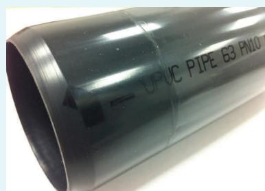
**Longitudinal reversion:** a sample of the product is immersed in an oven during 30 minutes at 150 °C: all tensions are released at this temperature considered as the beginning of fusion (fulfilled at 180 degrees). The product is then cooled at ambient temperature, and the deformation measured (shrinkage acceptable if smaller than 5%. This test helps to identify some processing abnormalities that might affect the pipe dimensions at long term, by evaluating the effect of heating on the pipe.
