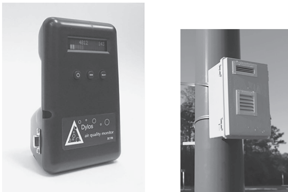
Figure 22.1 Dylos monitor and rain-proof enclosure
