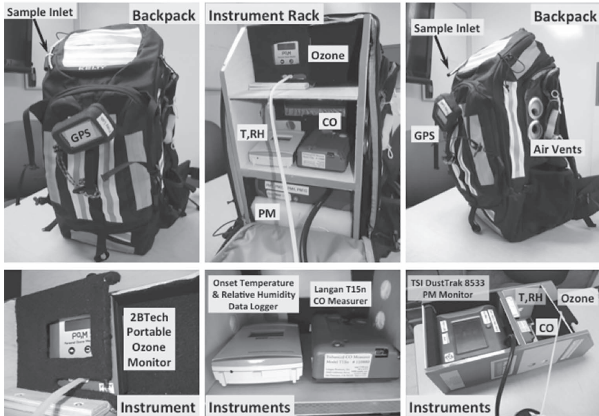
Figure 22.2 Instrumented backpack for Comparison of Air Pollution in Transportation microENVironments (CAPTEN) for particulate matter, carbon monoxide, ozone, temperature, humidity, and location
