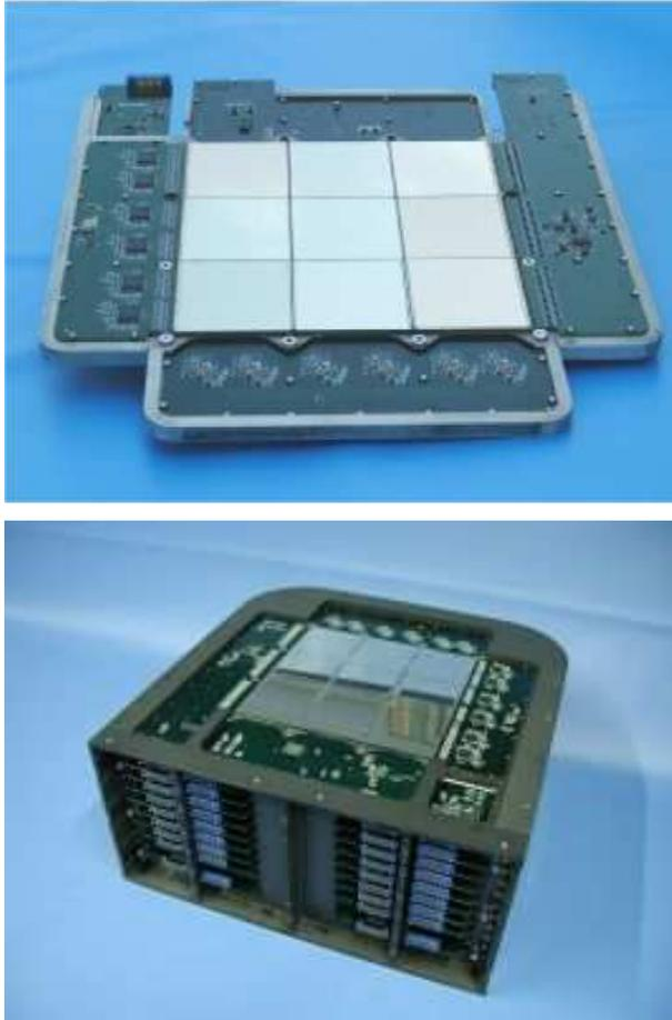
**Figure 2.6.** *Top:* picture of one *detection module* described in the text (see also section 3.4); the  $3 \times 3$  matrix of silicon strips with a size of  $(24 \times 24)$  cm<sup>2</sup> is clearly visible. *Bottom:* picture of the entire electromagnetic calorimeter [62].
