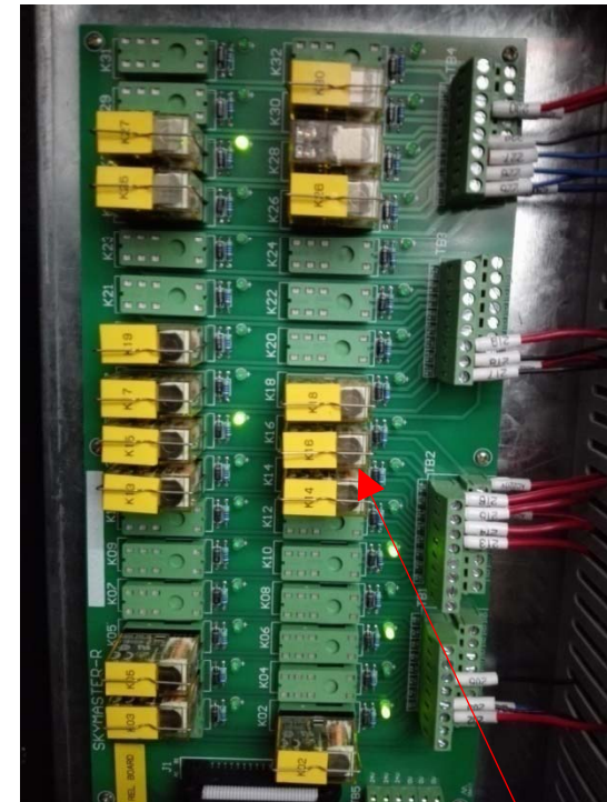
IDEC miniature relay from Japan
