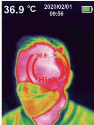
**HI/LO Temperature Alarm:** Central point temperature measurement, high/low temperature auto tracking and real-time temperature display.
