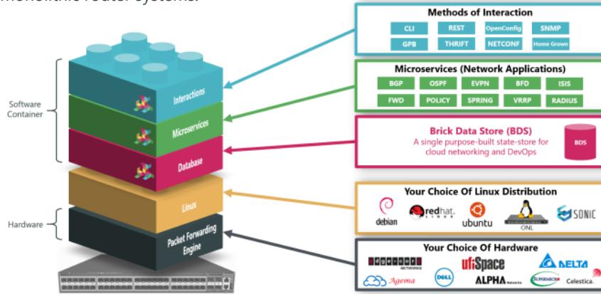
The RtBrick BNG is delivered as a Linux container and packaged for bare-metal switches within an Open Network Linux (ONL) installation for a seamless experience out-of-the-box. ONL handles peripherals such as LEDs, temperature sensors, and other platform management tasks. The entire networking stack, including the forwarding elements, is implemented in userspace as containerized processes.
