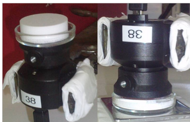
Figure 4. Measurement set-ups in reflection mode and sample presentation for the investigation. On the left, the lamps are pointing up and the 100% reflectance reference is placed inside a glass cuvette. On the right, the lamps are pointing down directly over the sample surface.
