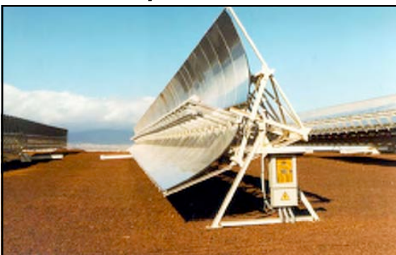
Fig.29 Example of a concentrator system. Source: The European Commission Directorate- General Energy and Transport
