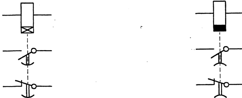
Figure 2 - Time delay relays and associated contacts.
