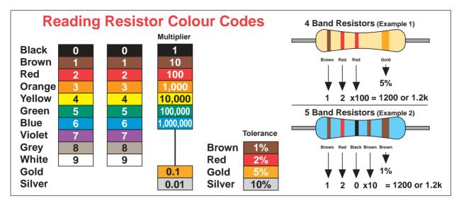
A resistor will limit the current flow through itself to a calculable value based upon its resistance and the applied voltage (see Ohm's Law). This means a resistor can be used to run a low voltage device from a higher voltage supply by limiting the required power to a predetermined level. Resistors are not polarity sensitive.
