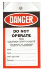
1. The student is to attach a DANGER TAG to the plug top of the project lead before proceeding with the allocated project. A danger tag must be attached to the plug top at all times when the lead is NOT plugged into the supply outlet. Plug tops or leads are not to be connected to the supply outlet WHILE A DANGER TAG is attached.
