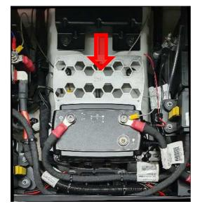
Carefully lift the CTEK120 up and slide the adaptor plate under, making sure that the large round holes go under the CTEK 120. The laser etched writing should face up and the plate is marked 120.
