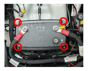
2. Using the T15 Torx bit, carefully loosen and remove the 4 x M4 screws that are holding down the CTEK 120. Carefully retrieve the rear bolts using long nosed pliers or magnetic pick-up tool.
