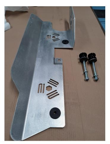
5. Now put the remaining large bushes in the four holes in the chassis rail you exposed by removing the rubber bungs in Step 1. The two smaller bushes go on the outside of the chassis rail, the two larger bushes go on the inside of the chassis rail. If in doubt, see the extra image under the heading **TOOLS & TIPS** on page 5.
