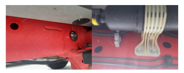
2. Unclip the fuel line on the front/engine side of the fuel filter. Place the fuel line on top of the clip and use a cable tie to secure it to the clip (so the fuel line does not rub on one of the bolts you will install in Steps 7 and 8).
