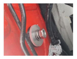
9. Now fully tighten the small single bolt on the underside of the guard (from Step 6). Next fully tighten the two longer 10mm chassis bolts.
