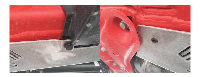
7. **Outer side of chassis rail:** now slide the two 10mm bolts with their washers through the chassis rail. Carefully thread the bolts through the two inner rail bushes.
