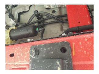
4. The two thin bushes should already be in the holes on the bottom side of the guard (near both logos). **Tip:** the logo is cut into the bottom of the guard in two places, allowing water to drain away. The logos also allow you to look for any dirt, mud or grass buildup and remove it.
