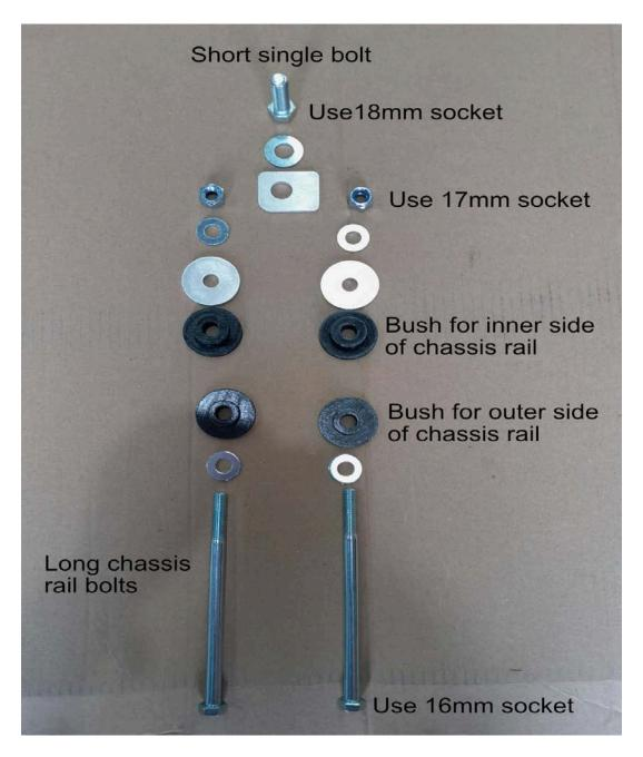
**Tip:** it is good practice to use a suitable <u>anti galling lubricant</u> on any bolt thread like those on the two long 10mm bolts.
