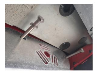
8. Inner (or filter) side of the chassis rail: Make sure the bolts are also threaded through the inner bushes. Ensure the bushes are still inserted in the chassis rail (adjust as required). Then put on the large aluminum washer followed by the small washer and finally the Nyloc nut.
