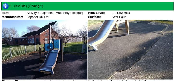
**Finding:** There are gaps opening between the surfacing and **Action:** Monitor for any further deterioration and repair as the edging surround or between the joints in the surfacing required
