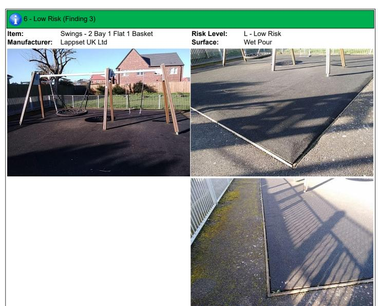
**Finding:** There are gaps opening between the surfacing and **Action:** Monitor for any further deterioration and repair as the edging surround or between the joints in the surfacing required
