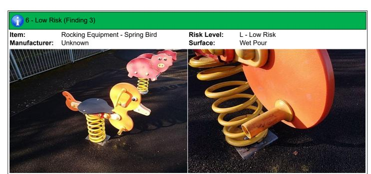
**Finding:** The end of handgrips and/or footrests have a cross **Action:** Monitor - No remedial work recommended section of less than 15cm2 and fail to meet the requirements of BS EN 1176 Part 6
