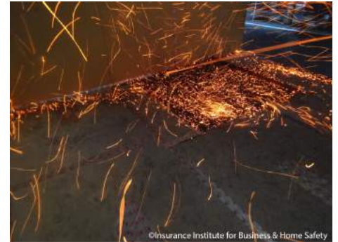
Wind-blown ember accumulation in deck board gaps at locations where deck boards intersected with the wood joists did not result in ignition of the higher-density wood-plastic composite deck boards.
