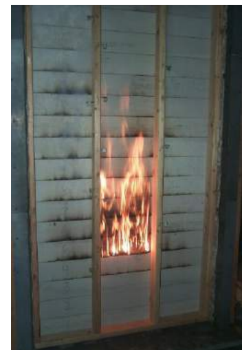
Flames from a gas burner on the opposite side of the wall resulted in flame penetration through a lap joint and into the stud cavity. The State Fire Marshal test method for combustible siding products consists of a flame impingement exposure, similar to that used in this test. As built, this siding product would not comply with Chapter 7A requirements. Source: firecenter.berkeley.edu/bwmg/siding-2.html
