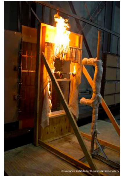
This cotton curtain ignited after both panes of a dual-pane window broke and fell out.
