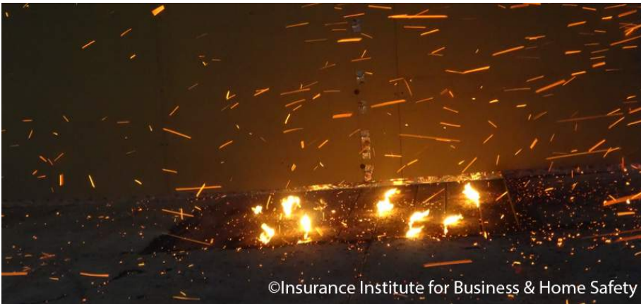
Wind-blown ember accumulation in deck board gaps at locations where deck boards intersected with the wood joists resulted in ignition of the deck boards.
