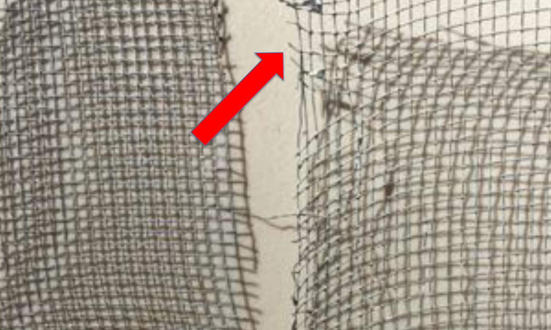
They aren't the same. Cheaper material (left, from PV store) has rough wire edges. The Hills Flat type (right) has smooth edges. Might make a difference on dust sticking to it?
