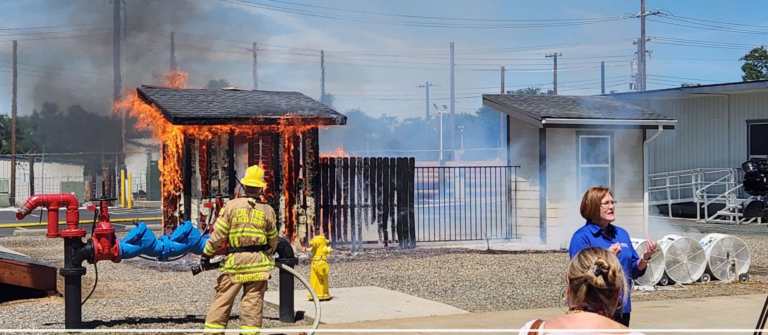
OSFM Zone 0 live fire demo | Sometimes reading about defensible space isn't enough. This live fire demonstration shows the impact a "Zone 0" noncombustible buffer of 5 feet around... | By CAL FIRE Facebook | Facebook
