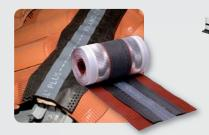
Material: Lateral laps made from mouldable aluminium and deformable up to 50%, containing water-repellent polypropylene in its central area and a double ventilation channel with a system of geometric openings for optimized ventilation (150 cm²/ml) while providing total protection against outdoor elements.
