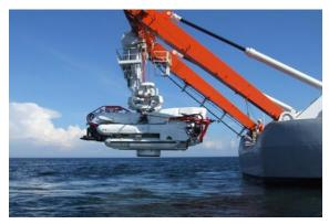
by two 25kW units, with a further four smaller units being used for positioning. It is the latest generation of rescue vehicle and has diverless recovery, fibre-optic data communications and a self-contained breathing system.
