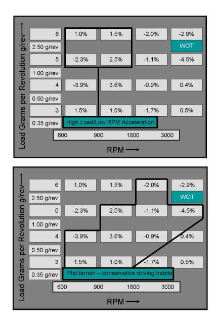
The important thing to remember here is that each cell is programmed with a formula to calculate injector pulse width under a variety of driving conditions. Long-term fuel trim values are learned for each load cell. Once a value is stored in a particular cell, then that fuel trim value will be applied the next time the vehicle enters that cell. The principles covered under Speed Density MAP fuel trim cells can be used for MAF fuel trim cell operation.
