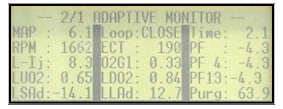
Time should be spent trying to relearn the PCM, performing a PCM reset, or disconnecting the battery to clear skewed information from the PCM. Later in this section, we will show how fuel trim cells operate, making it clearer how this affects PCM fuel trim operation.
