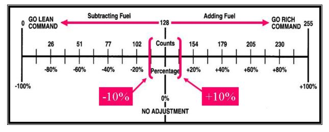
Regardless of the terms used for fuel trim, the PCM is always attempting to bring Short Term Fuel Trim as close to 0% as possible. In the real world, it is not expected that LTFT and STFT will both be near 0% because of the many engine operating variables, such as speed, load, temperature, fuel quality/volatility, etc.
