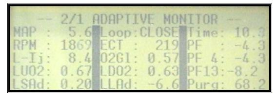
2. If the total Fuel Trim (LTFT + STFT) is more than 10%, the PCM begins changing Long Term Fuel Trim, attempting to bring Short Term Fuel Trim back to 0%. The following picture shows the PCM making a significant correction to the total fuel trim, now -1.4% (-14.1+12.7). This condition could occur immediately following a repair to the vehicle.
