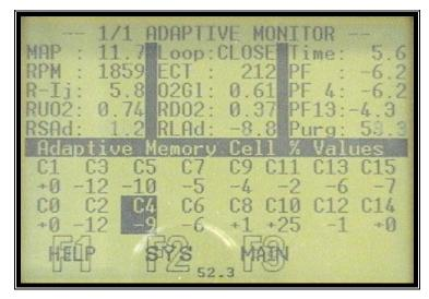
As the vehicle is accelerated, the Rpm/Load changes again, the PCM moves to another cell (C7) and trims LTFT by -4%. The PCM has moved to an upper cell because the engine Rpm is above 1984, and the load has increased.
