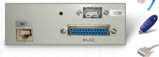
▪ The USB Port allows to upload and download through Flash drive.
