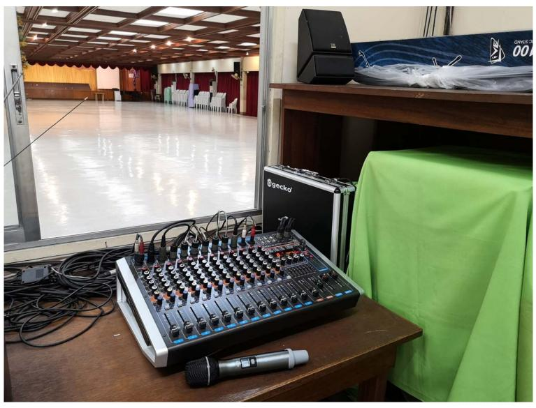
Driving these loudspeakers is the GECKO® EXODUS ATOM MXR 1208A 12-channel active C.R.I.S.T.A.L.® Audiophile mixing console, while connection of all the loudspeakers to the GECKO® EXODUS AT-OM MXR 1208A are done using the GECKO® TRUTH T2 audiophile-grade speaker cable terminated by the GECKO® OLYMPIAN series au-diophile-grade connectors.
