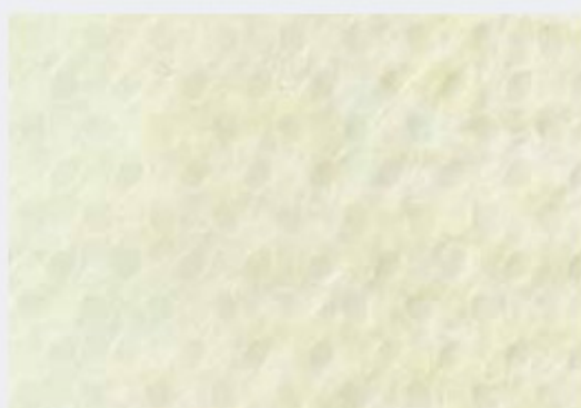
Soft Spunbond Polypropylene —used for inner and outer facings and for an extra layer of protection
