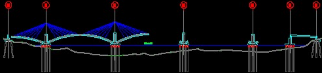
LONGITUDINAL SECTION PULAU BALANG -PENAJAM BRIDGE
