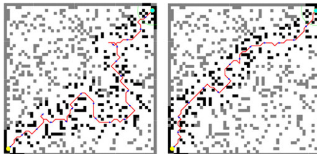
Fig. 3. Paths generated for different values of M in a randomized environment. The start point is the bottom left corner and the target is the top right corner. The left path was derived using M = 3 , the right path was derived using M = 25 .
