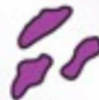
Irregular rodlike (chemical decomposition, mechanical comminution)
