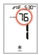
Use buttons to set the target set point for Cooling. Press "Fan" to advance to the next period.
