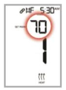
Use buttons to set the target set point for Heating. Press "Fan" to continue.
