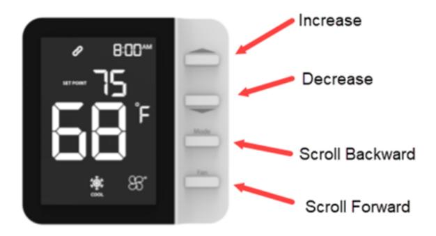
Use the "FAN" button to Scroll forward and the "MODE" button to backward through the available Parameter setup screens.
