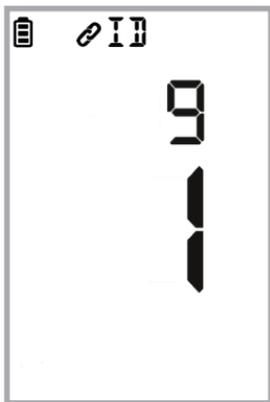
The module ID stops flashing, and 10-minute countdown timer begins.
