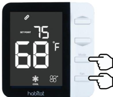
To access Parameters, hold down the **Mode** and **Fan** buttons until a beep sounds (3 seconds), then release.
