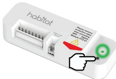
To initiate pairing, press and hold the **Pair** button on the HTM-01 Base Module until the LED flashes green (at least 5 seconds, but not more than 10 seconds). A continuous green LED indicates the base module is paired with the thermostat.
