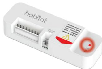
The LED on the module corresponding to the ID selected will begin flashing red for 10 minutes. If "All" is selected, the LEDs on all connected modules will flash red.
