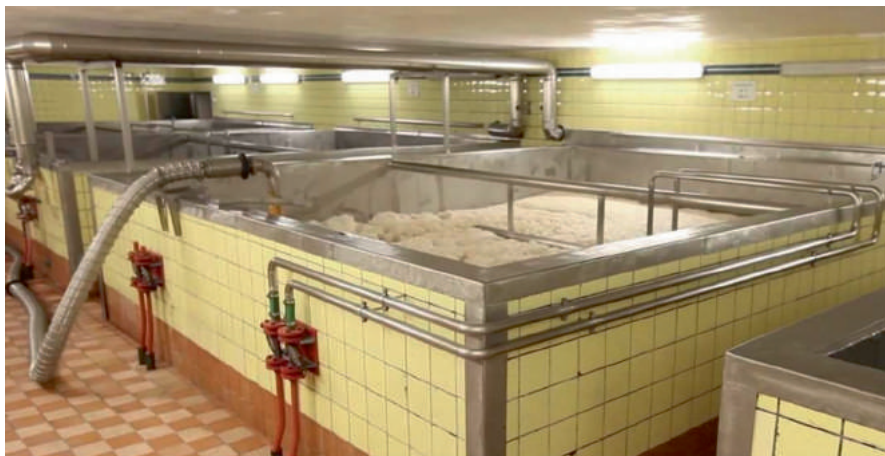
Fig. 11.3 Square tank for wheat beer fermentation
