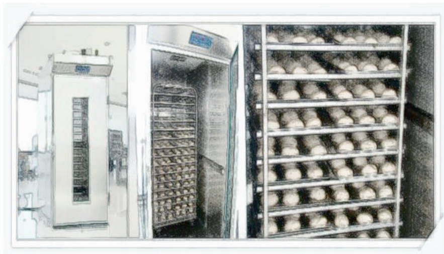
Fig. 11.6 Stainless steel automatic dough retarder proofer
