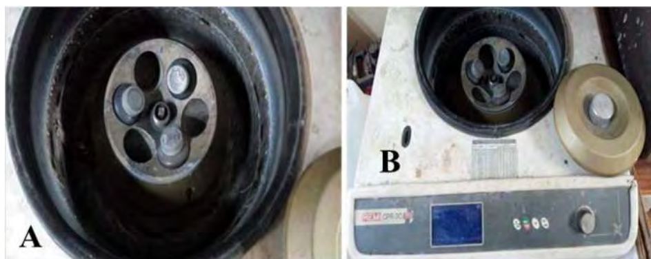
Figure 1. Image of the R - 236M rotor (A) and the laboratory fixed-angle conical rotor centrifuge (B).
