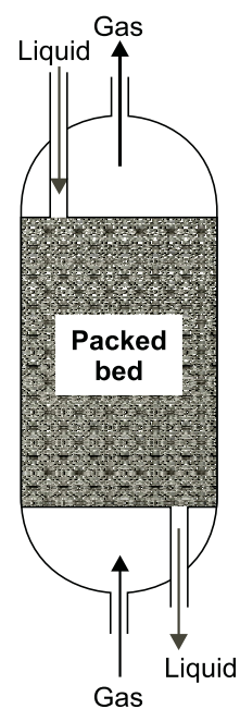
Figure 3. Packed bed bioreactor with the counter current flow
